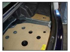
**STEP 2**Remove both of the hardboard floor inserts
